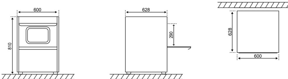
Dishwasher foot height is 20 mm. Foot height cannot be adjusted. Maximum inlet opening height is 380 mm.
